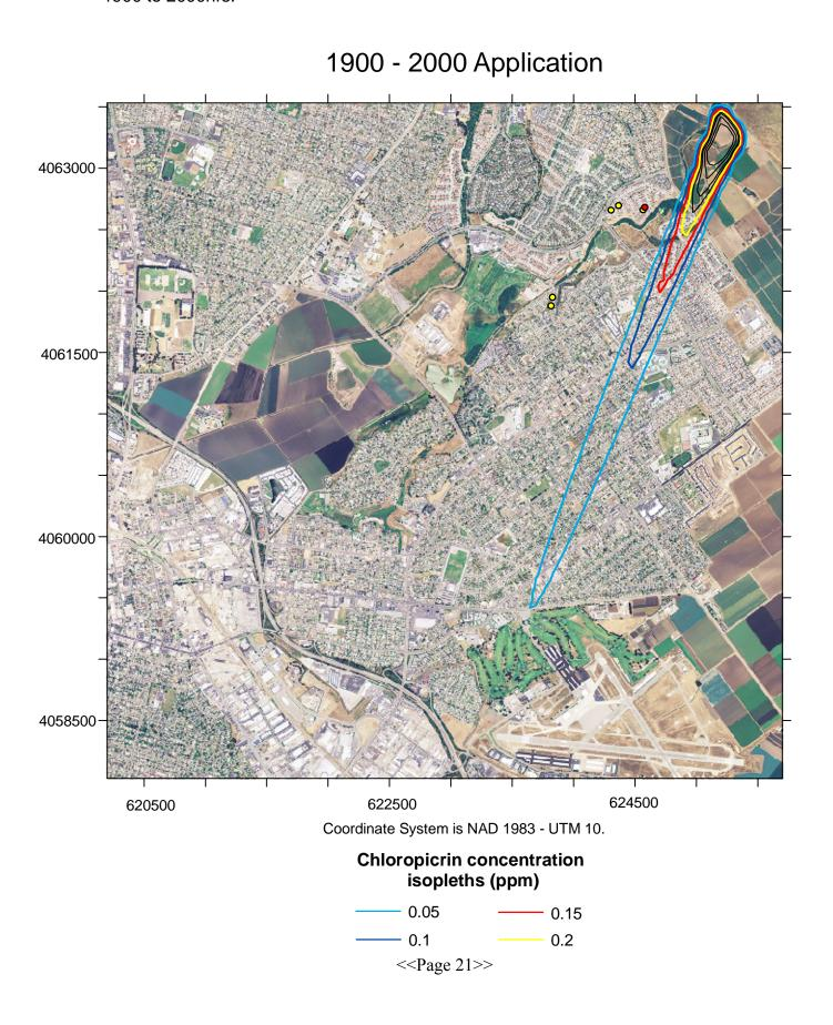
Figure 9. Estimated chloropicrin air concentrations associated with the drip application made to Block 20 of Daren's Berries, Salinas, California. Chloropicrin air concentration estimates are for the interval 2000hrs to 2100hrs (PDT) October 5, 2005. The yellow dots show locations of 911 calls received during the hour.
