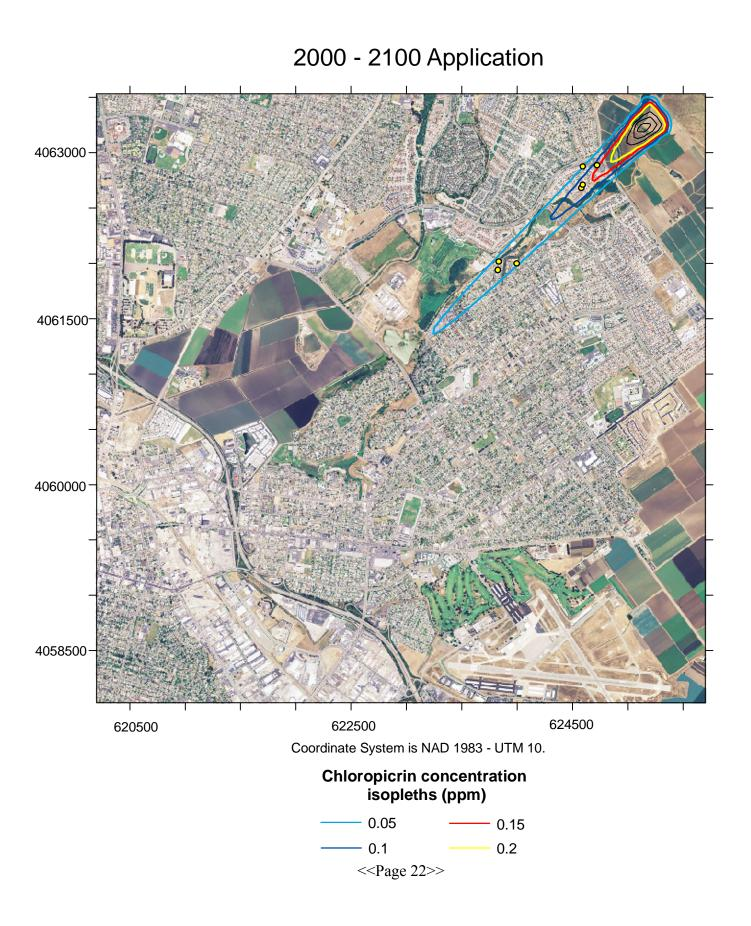
Figure 10. Estimated chloropicrin air concentrations associated with the drip application made to Block 20 of Daren's Berries, Salinas, California. Chloropicrin air concentration estimates are for the interval 2100hrs to 2200hrs (PDT) October 5, 2005. The red dot shows the location at 2158hrs of the officer at the corner of Boronda and Constitution. The yellow dots show locations of the 911 calls received during the hour.
