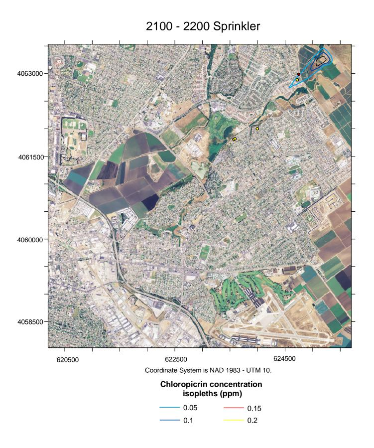
Figure 8. Estimated chloropicrin air concentrations associated with the drip application made to Block 20 of Daren's Berries, Salinas, California. Chloropicrin air concentration estimates are for the interval 1900hrs to 2000hrs (PDT) October 5, 2005. The red dot shows the location of the first 911 call received at 2015hrs. The yellow dots show locations where after the fact interviews indicate residences have been affected during 1900 to 2000hrs.
